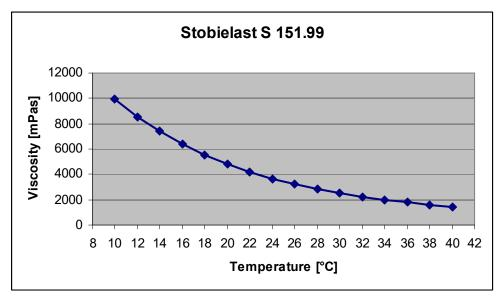
Diagram : Viscosity of Stobielast® S 151.99 depending on temperature; measuring system (4/100) Brookfield CAP 2000L
